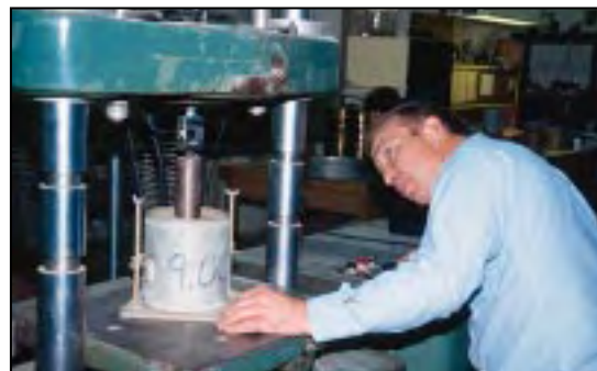
Figure 1. A technician applies load to a compacted soil specimen in a CBR mold. Specimens were loaded with and without sand layers to determine the effect of differing sand-layer thicknesses.
